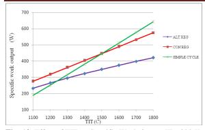
Fig: 12. Effect of TIT on Specific Work Output [T<sub>1</sub>=300 K,
