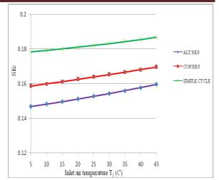
Fig: 16. Effect of the Inlet Air Temperature on Specific Fuel Consumption [TIT = 1500  $^{0}$ C, r = r<sub>opt</sub>]
