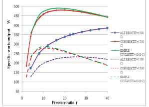
Fig: 7. Effect of Pressure Ratio on Specific Work Output with TITs  $[T_1=300 \text{ K}, \text{ E}=0.8]$
