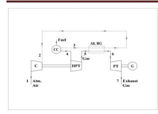
**Fig: 3.** Schematic Diagram of Gas Turbine with Alternative Regeneration Cycle
