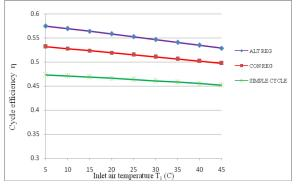
Fig: 14. Effect of the Inlet Air Temperature on Efficiency  $[TIT = 1500 \ ^{0}C, r = r_{opt}]$
