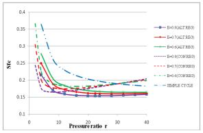
**Fig: 10.** Effect of Pressure Ratio on Specific Fuel Consumption with Effectiveness  $[T_1=300 \text{ K}, \text{TIT}=1500 \ ^0\text{C}]$
