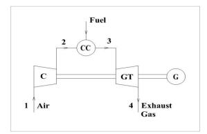
Fig: 1. Schematic Diagram of Simple Gas Turbine Cycle
