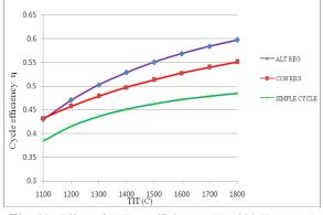
**Fig: 11.** Effect of TIT on efficiency  $[T_1=300 \text{ K}, r = r_{opt}]$
