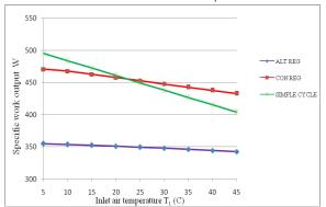
Fig: 15. Effect of the Inlet Air Temperature on Specific Work Output [TIT =  $1500 \ ^{0}$ C, r = r<sub>opt</sub>]
