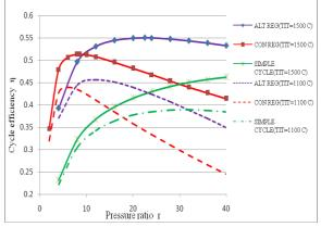
Fig: 5. Effect of Pressure Ratio on Cycle Efficiency with TIT  $[T_1=300 \text{ K}, \text{E}=0.8]$
