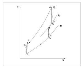
Fig: 4. Schematic Diagram of T-s Diagram of Alternate Regeneration Cycle
