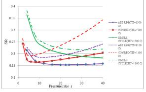
**Fig: 9.** Effect of Pressure Ratio on Specific Fuel Consumption with TIT [T<sub>1</sub>=300 K, E=0.8]
