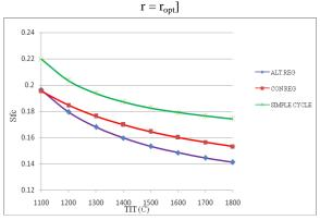
Fig: 13. Effect of TIT on Specific Fuel Consumption  $[T_1=300 \text{ K}, r=r_{out}]$
